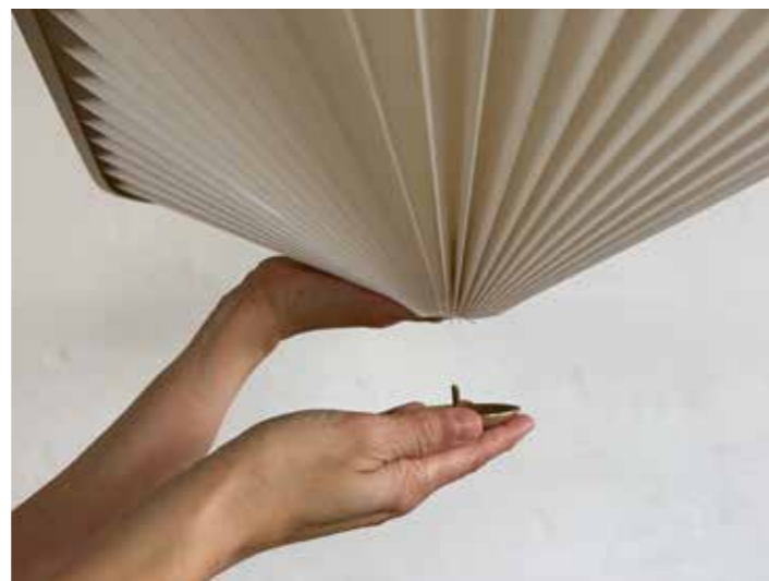
71. Once all the pleat tips are sitting on the ledge of the frame, hold the shade in place while another person hands you the metal bottom.
